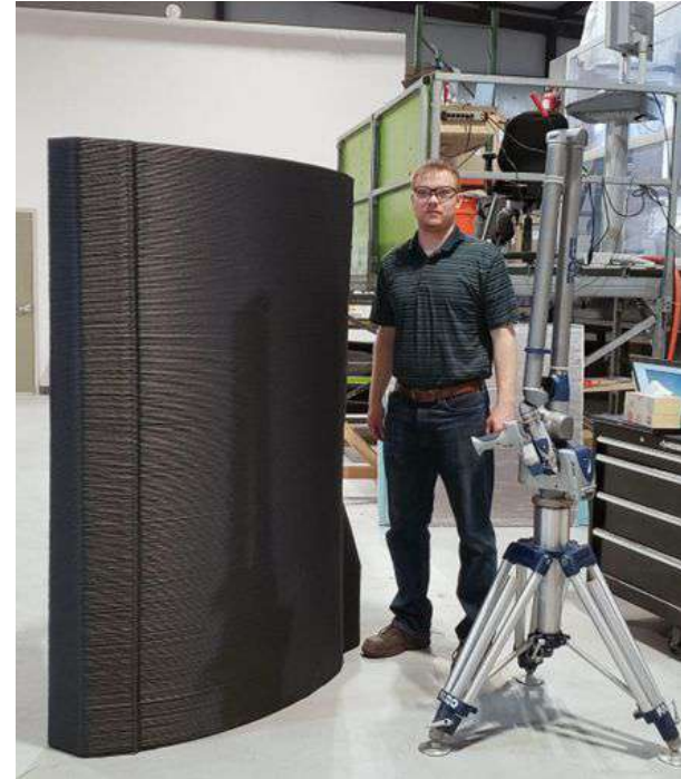
3D Printed Layup Mold - No master needed.
