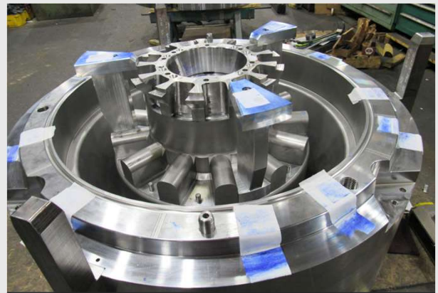
64" diameter, precision turning and machining
